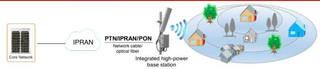
In rural and suburban areas, the wireless network coverage is relatively wide, but the users are less fixed than the fixed ones. By deploying LTE integrated high-power base stations in a town or natural village, the signal coverage in a small area can be achieved, reaching low Investment in rural 4G wireless access.
